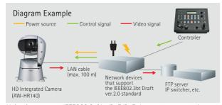
Hubs that support IEEE802.3af/at(PoE/PoE+) are not supported. \* Abbreviation of Power over Ethernet Plus Plus.
