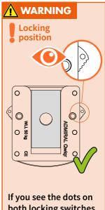
both locking switches, the Qwiqr is locked.
