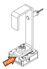
Step 1 Push the clamp part against the spring block.
