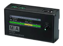
Are you looking for a DMX node in your theater, TV studio, house of worship or other installation? The grandMA3 onPC xPort Nodes DIN-Rail are the perfect solution for you! The nodes fulfill two different tasks: They convert Ethernet data to DMX and they can add parameters to your grandMA3 onPC system.
