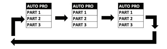
The Secondary unit receives data from the Primary unit according to the group that the Secondary unit was assigned to. For example, suppose we have a unit that has been assigned as a "Secondary 1" unit. Upon receiving the 3-part Auto Program from the Primary unit, the Secondary 1 unit will implement Part 1 of the Auto Program, while ignoring Part 2 and Part 3.
