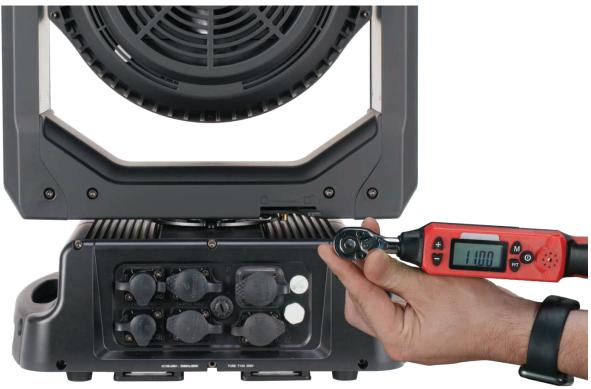
The hex-head screws holding the panels MUST be tightened with a torque wrench (Torque Wrench Not Included.
