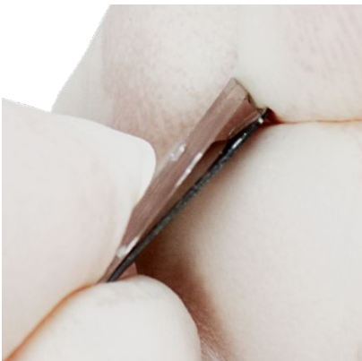
14. Carefully remove the retaining ring washer attached to the GOBO.
