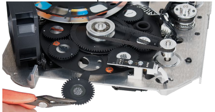
11. Carefully lift the GOBO Holder up and out from the GOBO wheel using small needle nose pliers.
