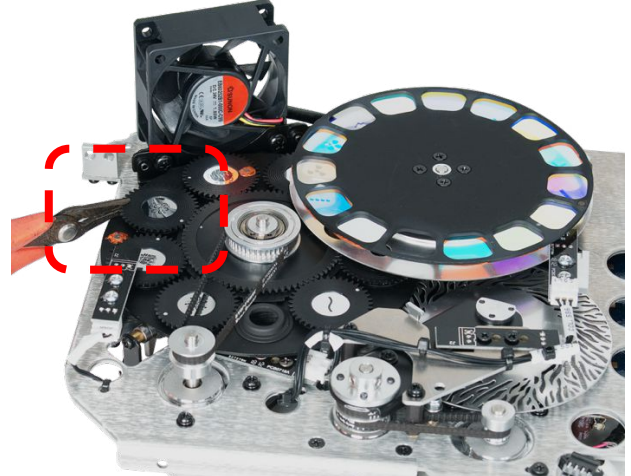
10. Place the effect module on firm clean surface and locate GOBO to replace.
