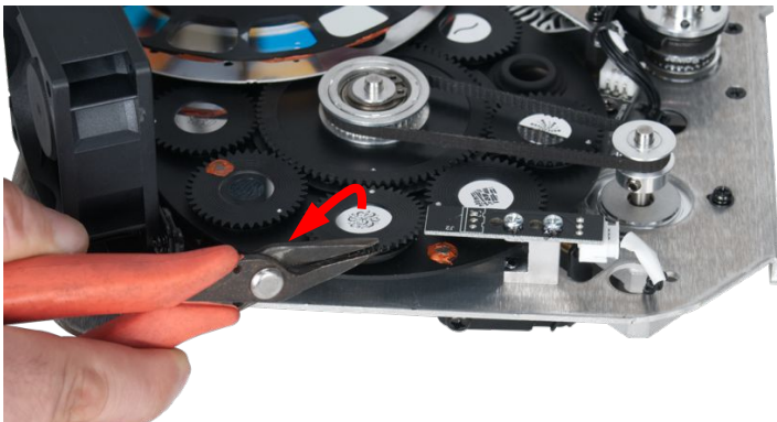
11. Carefully lift the GOBO Holder up and out from the GOBO wheel using small needle nose pliers.
