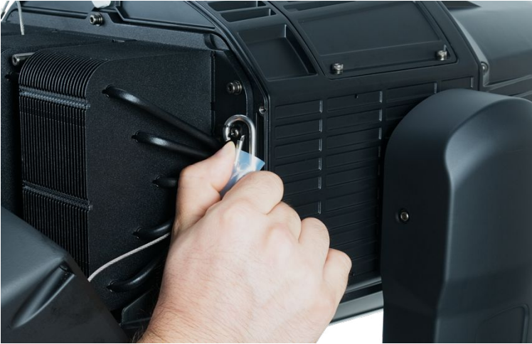
4. Unclip the rear cover safety cable.
