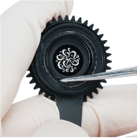
12. Carefully remove retaining spring.
