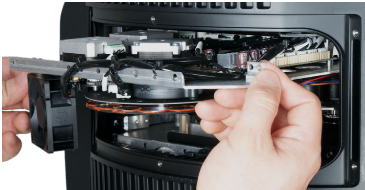
9. Carefully remove the effect module from fixture.
