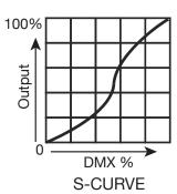
The S-Curve Dimmer Curve is ideal for controlling a blinder-type fixture, as it features a smooth bottom and has no harsh reduction in lighting intensity when fading down from 100% output. When operating in a DTW-enabled setting with manual fader control, the S-Curve will provide the most natural feel.
