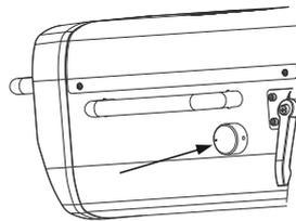
The intensity of the fixture is set with the Dimmer Encoder.
