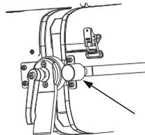
The manual zoom of the fixture can be adjusted with the Zoom Slider.
