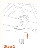
Attach the coupler to the supporting structure.
