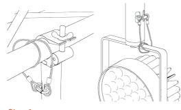
Step 1 Remove the safety cables from both ends.
